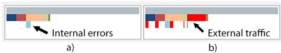
Figure 5.8: a) Application of INVITE (blue), ACK (bordeaux), and error messages (orange/blue). b) Messages in red represent external traffic.
