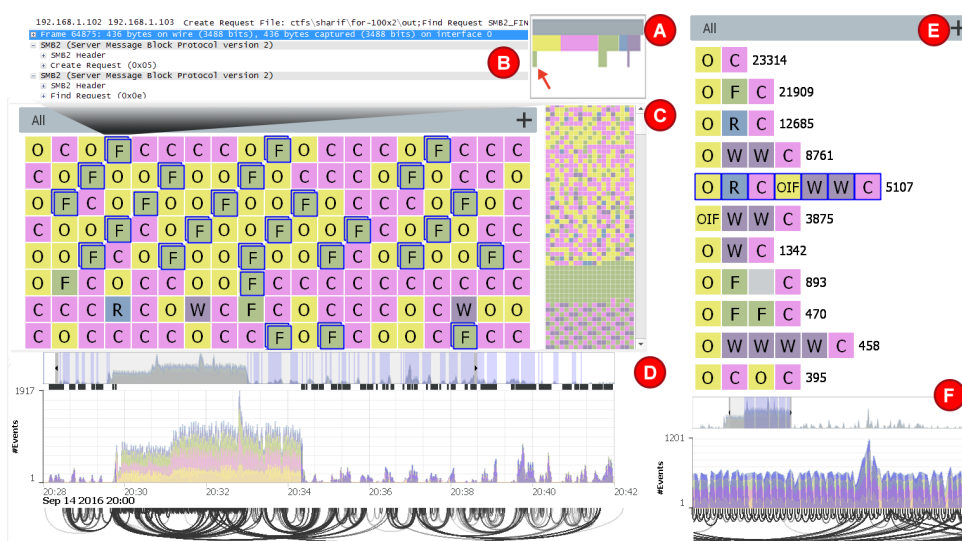
Figure 7.12: A) The icle plot shows that some CryptX packets are both Open and Find requests. B) Inspection with Wireshark. The minimap (C) and line chart (D) show that compound requests are sent before directory traversal and outside the encryption phase. E) Grouping the traffic by smb2.filename shows that files are overwritten. F) During encryption files are opened and closed sequentially.
