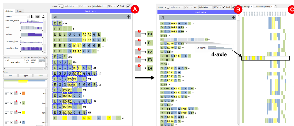
Figure 6.6: A) Inspection of 4Axle truck and bus patterns. The travel patterns by buses are highlighted in blue. B) Application of detailed ruleset. C) The alignment of bus and truck traffic shows a suspicious long sequence (indicated by the black box).
