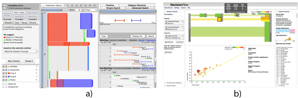
Figure 2.17: a) EventFlow [223] is an extensive novel tool to summarize univariate event sequences, search for temporal patterns, and apply data transformations to gain new insight in event collections. b) Decision-flow [122] enables high-dimensional analysis by introducing a milestone-based aggregate data structure and corresponding temporal query methods.
